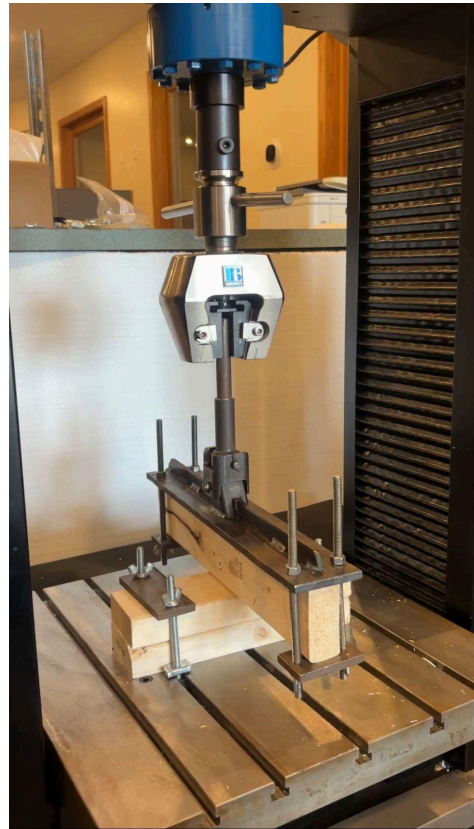
Fig. 2 Designed steel fixture and truss chord
