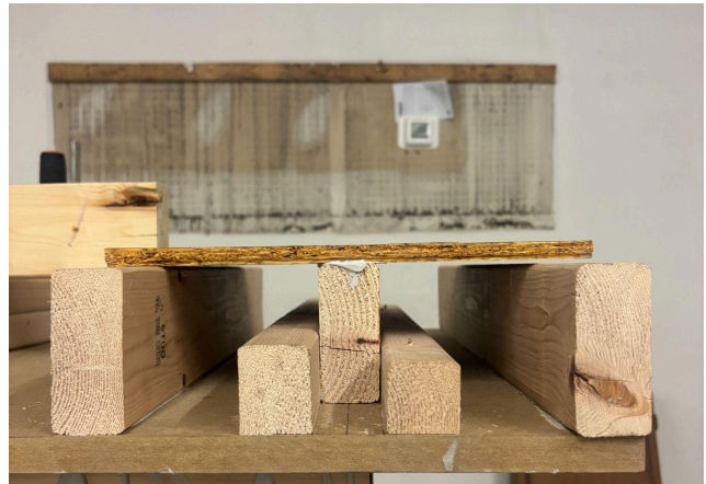
Fig. 2 Wood channel for rafter to sheathing adhesion
