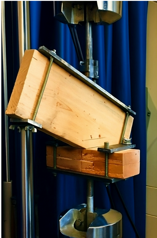
Fig. 1 Designed steel fixture and bird mouth
