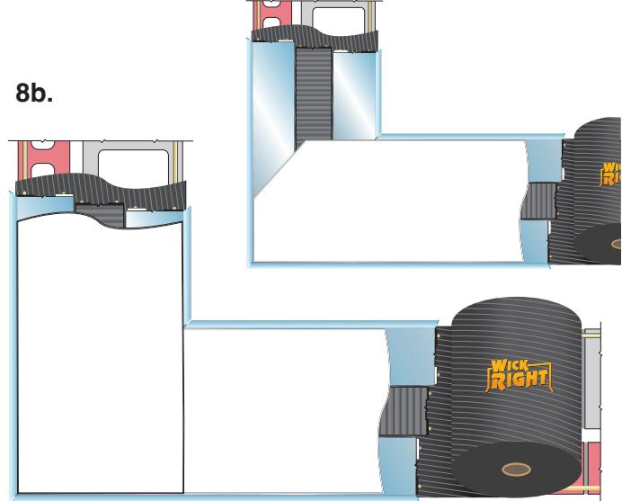
**9.** Re-install capstones – Typical size capstones should be re-set in a heavy bed of polyurethane sealant as shown. We use Sika brand.
