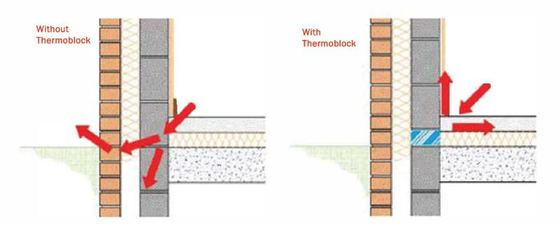
Foundation and roof perimeters are both locations in the building thermal envelope where heat is lost due to thermal bridging. Thermoblock® reduces energy lost by thermal bridging, providing continuous insulation at the base of a wall, slab edge or roof parapet intersection where insulation is normally interrupted. Thermoblock® has a thermal conductivity 2 times lower than timber and 30 times lower than concrete.
