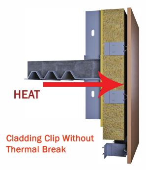
The purpose of a thermal break is to reduce the impact of thermal bridging by preventing conductive heat flow through the building thermal envelope. Thermal breaks also help to keep surface temperatures within the thermal envelope above the dew point. This eliminates potential condensation risk.
