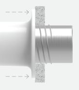
3 Firmly hold the O-in<sup>™</sup> installation housing against the drywall surface in order to maintain the tool's perpendicularity. Push and rotate in a clockwise direction until the O-in™ installation tool adapter sleeve is completely screwed into the drywall. Remove the installation tool.
