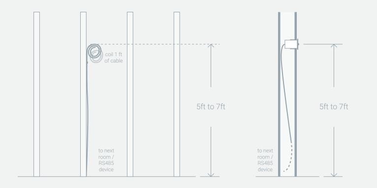
Before drywall is installed, run two wires in a daisy chain configuration through the studs.
