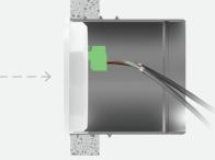
(i) The plastic protection cap holds the wired connector in place and protects it from dust and debris during all the construction phases.
