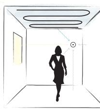
People typically respond to thermal discomfort by continuously readjusting their thermostat. The problem is that an air based thermostat never represents the real human thermal exchange. mSense comfort sensor is an essential element of a climate control system especially in presence of radiant celling panels but also in conventional radiant floor and air systems.
