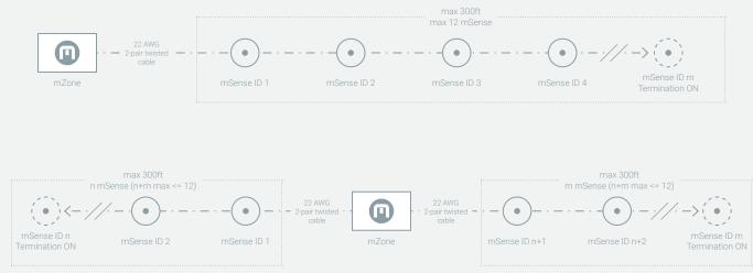
When the mSense sensors are locally powered, the maximum number of physical mSense devices connected to the serial bus is 64, unless further restricted by other third party devices present on the same bus. Bus extenders can be used to overcome the 64 device limitation (not supplied by Messana).
