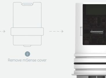
The Slave address must be manually configured through the dip-switch SW1. The dip-switch can be accessed by removing the mSense top cover as show in the pictures above.
