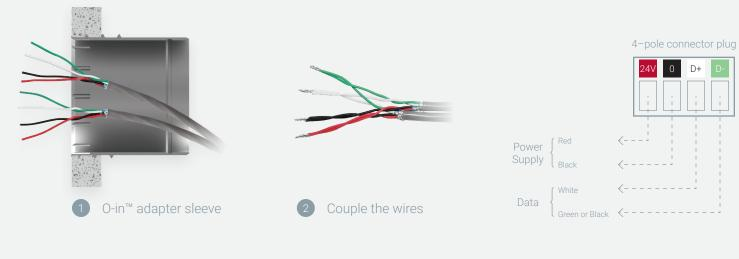
Insert the plug connector into the O-in<sup>™</sup> protection cap.
