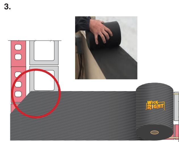
**4a.** Start at a corner, cut membrane as shown here. Overlap membrane layers as shown here. Apply a 3/8" bead of sealant on the underside of the membrane being placed on top along the interior and exterior edges.
