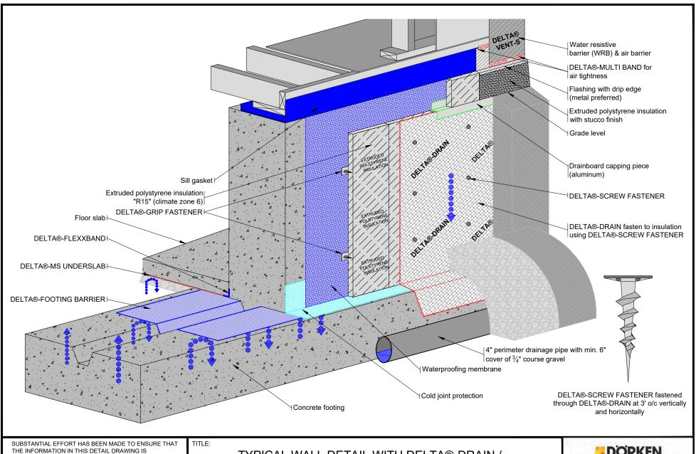
TYPICAL WALL DETAIL WITH DELTA®-DRAIN / DELTA®-FOOTING BARRIER / EXTERIOR EXTRUDED POLYSTYRENE INSULATION CLIMATE ZONE 6 (2012 IECC)
