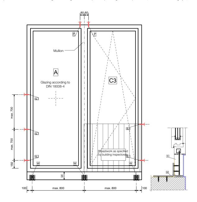
P = fixing in the anchor base with blaugelb Protect and blaugelb Frame Screws Fix FK-T30 7.5  $\times$  L
