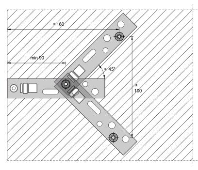
1x Protect with adjusting screw and 2x Protect without adjusting screw – angle from horizontal of  $\leq 45^{\circ}$  and  $\geq 100$  mm 3 blaugelb Frame Screws Fix
