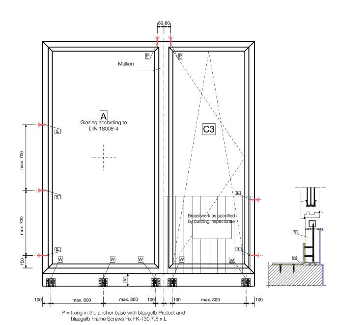
This schematic diagram highlights only the safety-relevant fastenings in accordance with the ETB guideline "Components providing fall arrest protection"
