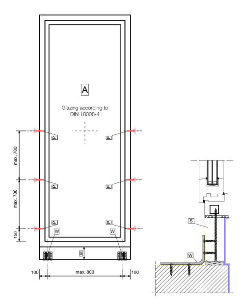
P = fixing in the anchor base with blaugelb Protect and blaugelb Frame Screws Fix FK-T30 7.5 x L
