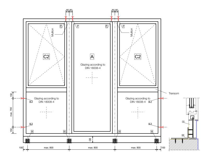
P = fixing in the anchor base with blaugelb Protect and blaugelb Frame Screws Fix FK-T30 7.5  $\times$  L
