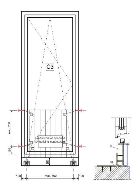
P = fixing in the anchor base with blaugelb Protect and blaugelb Frame Screws Fix FK-T30 7.5 x L
